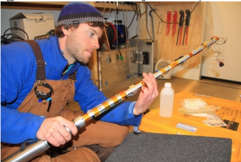
Dan: Dan repairs the sonic logger in the drillers workshop.
