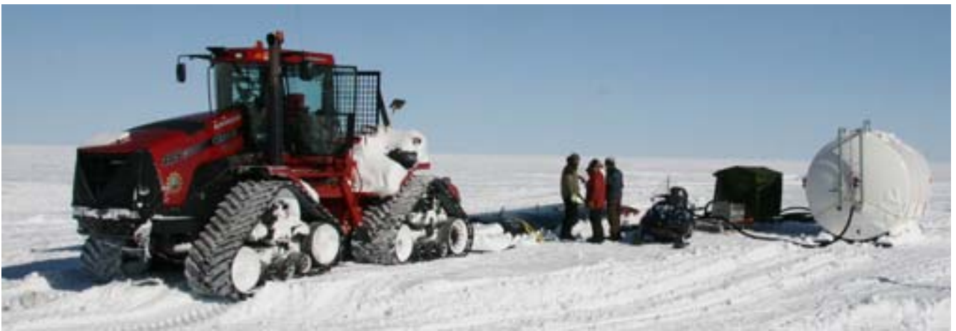
Fuel transfer: Our diesel fuel pump was hard at work transferring fuel from tractor train bladders to NEEM tanks.
