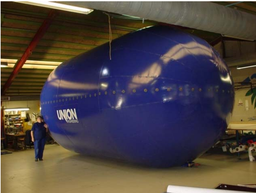
A smaller version of the inflatable tank that will be used to cast the trench.
